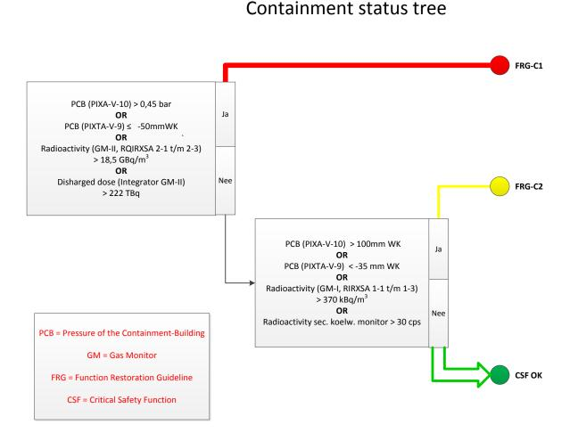
Fig 1. Example of a status tree for the containment function
